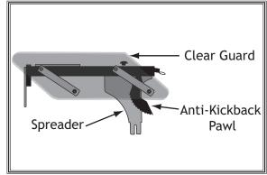
**Figure 37.** Blade guard assembly components.
